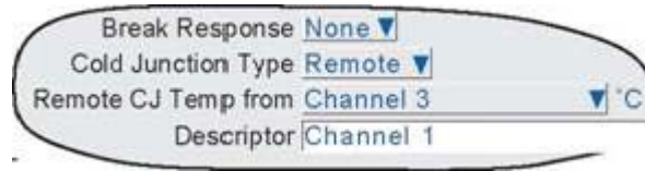
Figure 61. Remote Cold Junction Compensation
