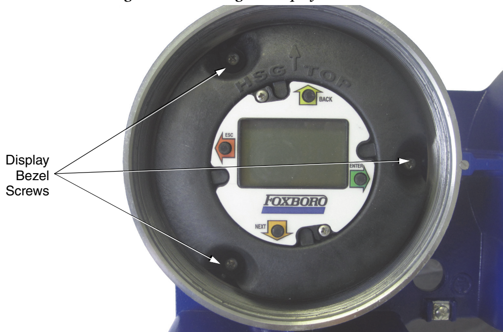
Figure 49. Loosening the Display Bezel Screws
