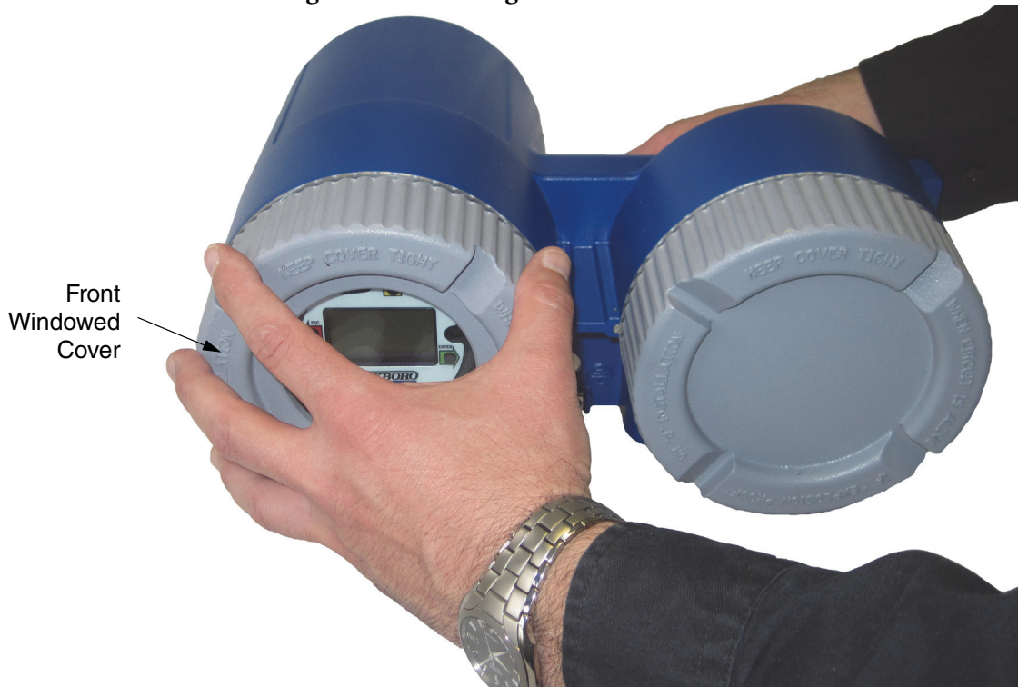
Figure 48. Removing the Front Windowed Cover
