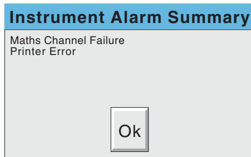
Figure 3.1.4b Typical Instrument alarm summary display
