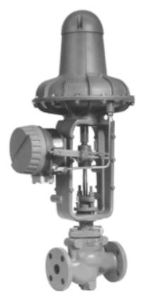
The Foxboro<sup>®</sup> brand E69P Valve Positioner, mounted directly on a pneumatic valve yoke, converts a standard direct current input signal to a proportional valve stem position. It eliminates the need for a separate converter plus a separate positioner. As symbolized by the "CE" Logo marking on the product, these valve positioners conform to the applicable European Union directives.
