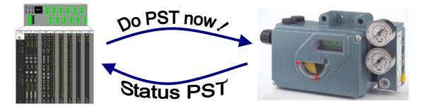
The communication protocol is used only to send information to a PC or a DCS in charge of the diagnostic and predictive maintenance.
