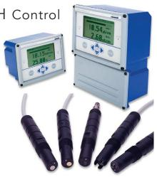
Invensys Foxboro® 875PH intelligent analyzer and DolpHin sensors are a proven system for demanding pH measurement applications. The 875PH analyzer provides ease-of-use advantages such as two alarm relays, two 4-20 mA outputs, and an RS-232 serial port for remote configuration. The Foxboro DolpHin™ pH sensors utilize a proprietary glass formulation for high temperature service, allowing use in applications with temperatures as high as 250° Fahrenheit (121° Celsius).
