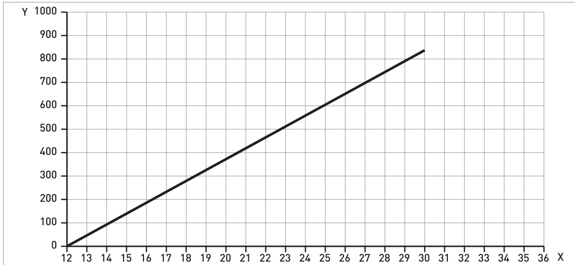
Figure 2-3: Minimum power supply voltage for an output of 21.5 mA at the terminals (Non-Ex and Hazardous Location approval (Ex i / IS))
