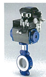
Wafer 1.0619 (WCB) PTFE/PFA, pneum. actuator and E/P positioner
